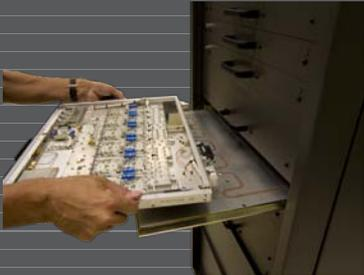
The concept behind Cool-Dock is a superior cooling configuration which utilizes no hose couplings, or water connections which need to be disconnected in order to service the transmitter modules. This innovation eliminates connection points along with potential for leaking or mechanical failure. As an added benefit, active device cooling is superior to traditional designs. The result is better performance and higher reliability.
